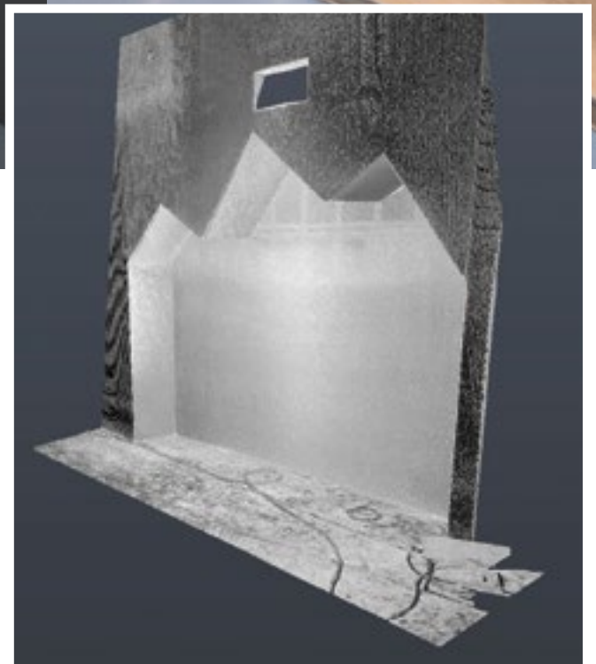
Above: A detailed laser scan captured the exact shape of the recessed seating areas along the building's curved main hallway. With this precise information, our wood shop was able to fabricate the materials offsite and complete installation smoothly and efficiently.
